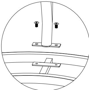
STEP 3 - Attach centre ring (5) using 6 x bolts (B) and 6 x nuts (C). Tighten all fixings.
